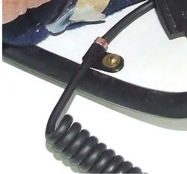
Picture 6. The helmet lining pulled back to show the communication cord attachment.
