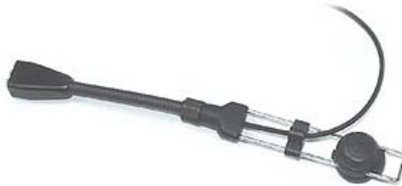
Picture 4. Microphone boom viewed from the outside (the wire must be on the outside of the boom, and the microphone securing screws must face the inside of the boom – towards helmet)
