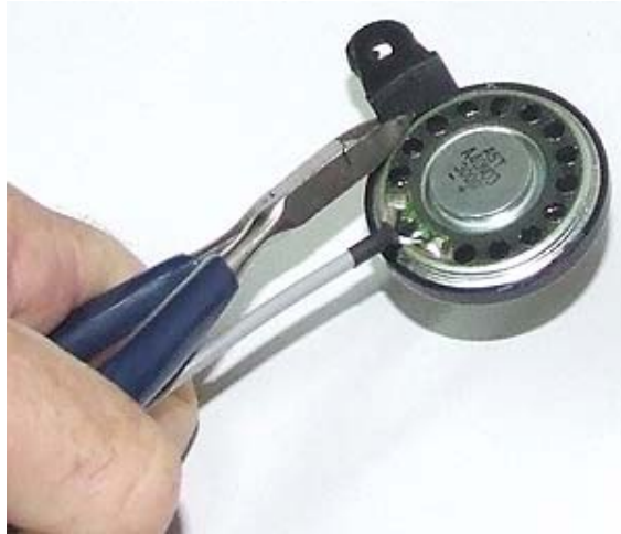
Picture 1. Trimming off earphone speaker mounting lugs
