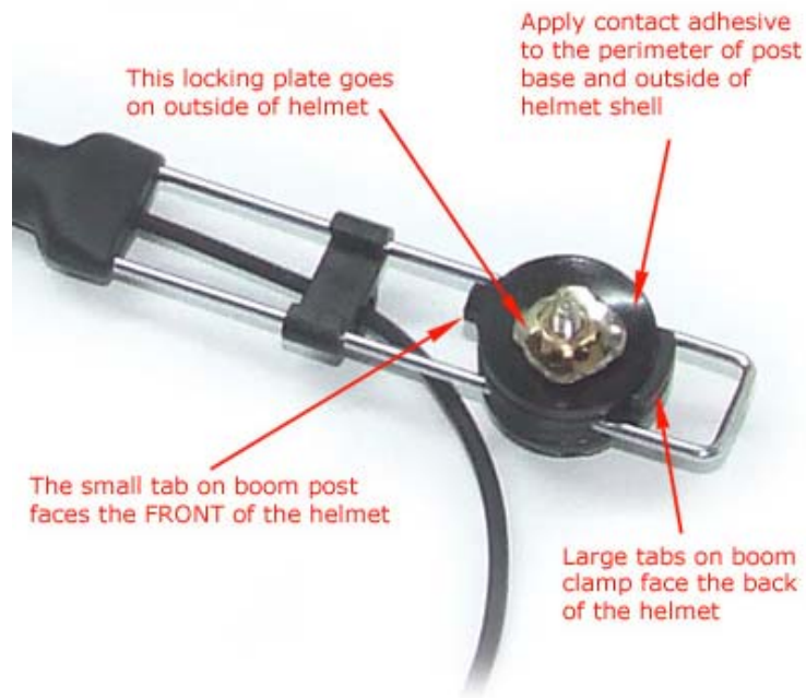
Picture 3. Microphone boom post detail (the nut is removed prior to installation)
