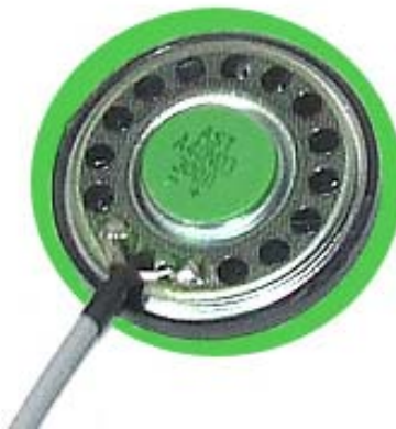
Picture 2. Earphone speaker safe gluing areas
