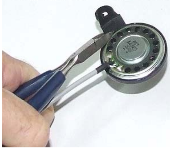
Picture 1. Trimming off earphone speaker mounting lugs
