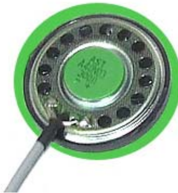
Picture 2. Earphone speaker safe gluing areas
