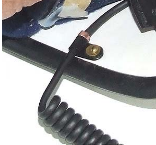
Picture 3. The helmet lining pulled back to show the communication cord attachment.
